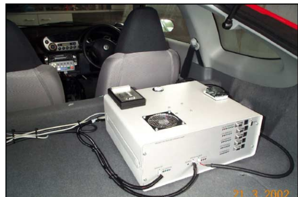
Fig. 21. Data logger in the Insight .
