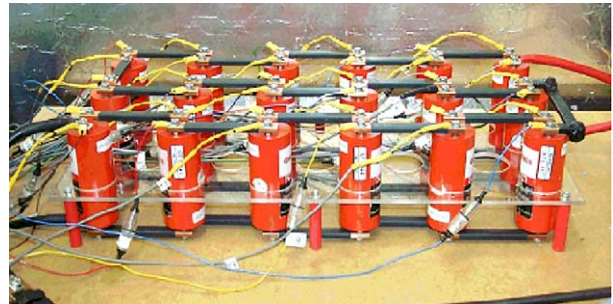
Fig. 10. A pack of 18 dual-tab cells under cycle test.
