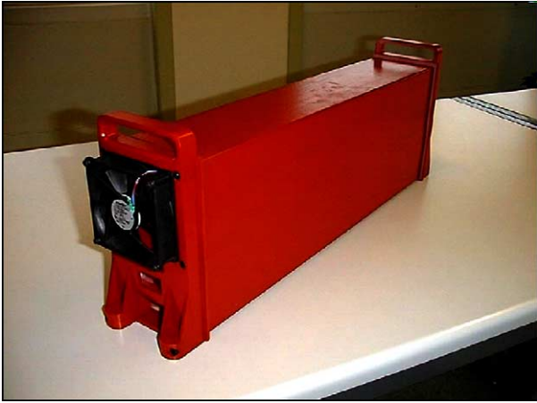
Fig. 19. Prototype module casing with cooling fan.
